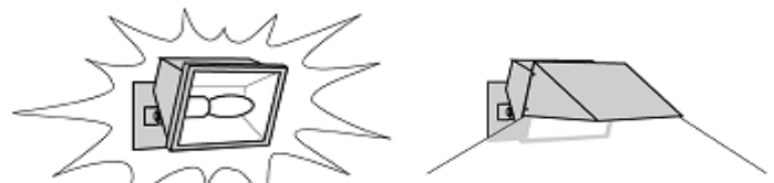
Glare from unshielded floodlight
