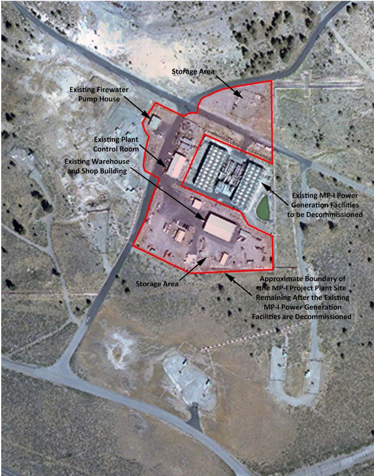
Figure 12: MP-I Project Plant Facilities and Areas that Would Not be Decommissioned
