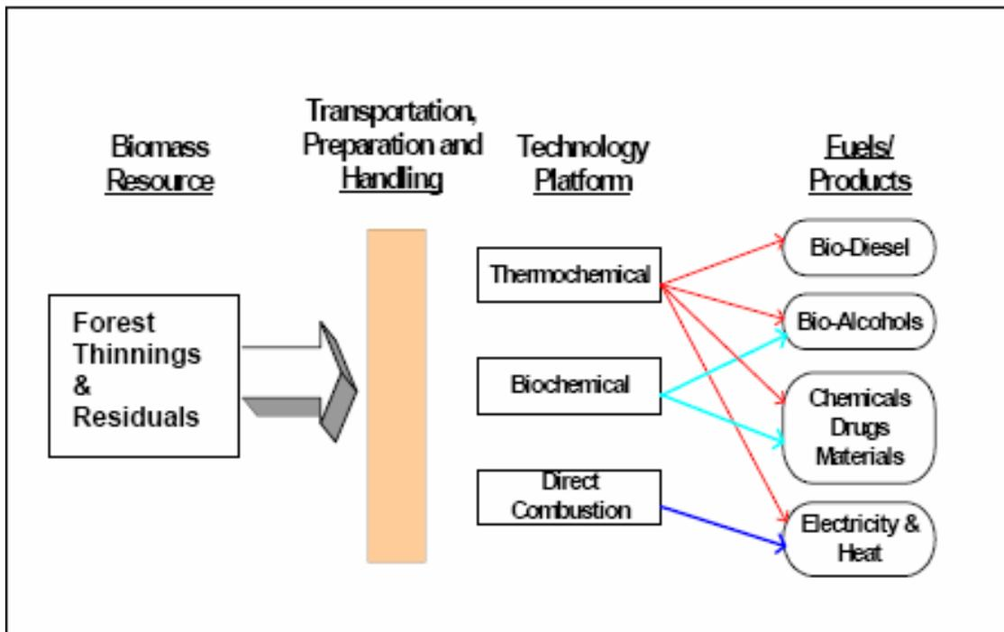
Figure 3. Existing and emerging biomass utilization technologies
