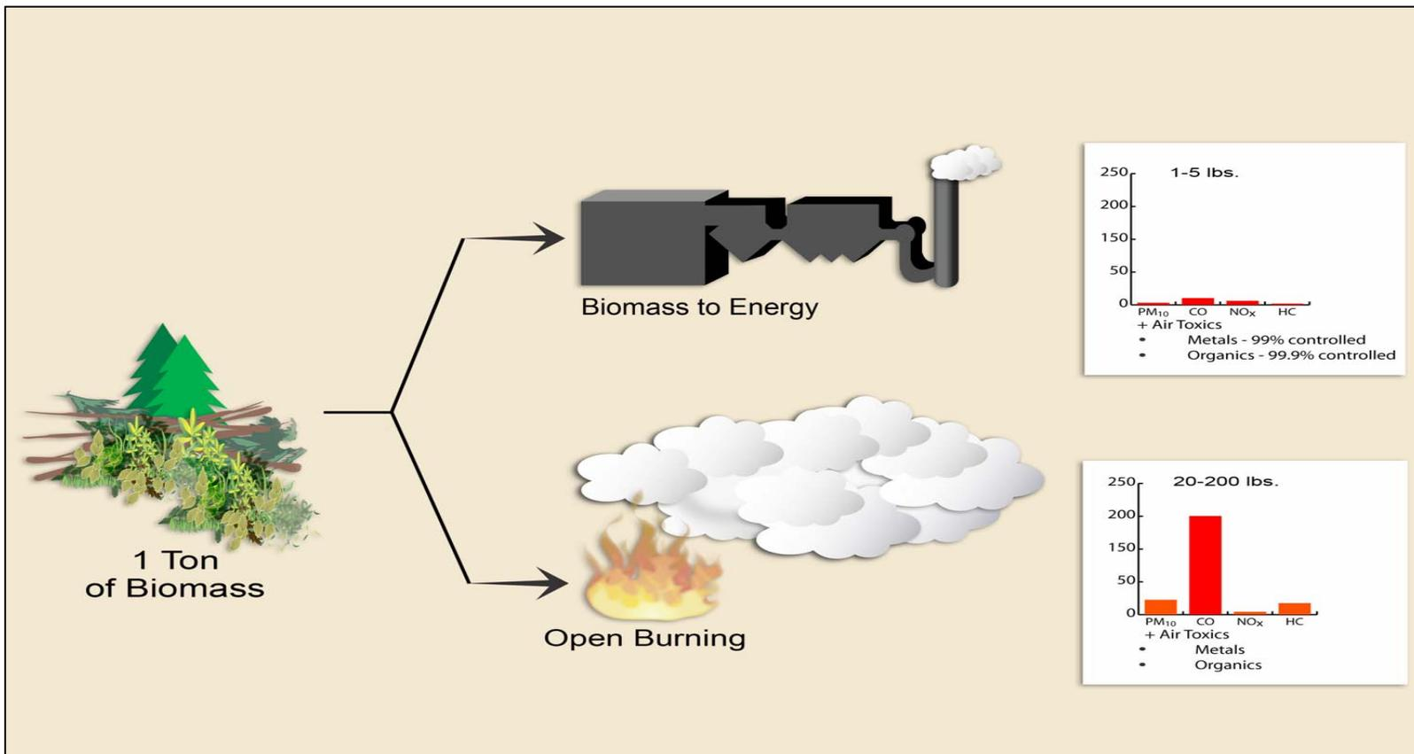
Figure 10. Difference in emissions between open and controlled burning
