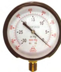
At the fabricator's shop, the testing vacuum in the interstice should be retained for a minimum of 24 hours at -25" Hg. Many tank manufacturers keep the vacuum at this level for 48 hours--my experience says the longer the better.
